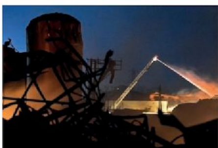
Nitrates can decompose explosively to cause a large amount of damage, as shown by the remains of this fertiliser factory
