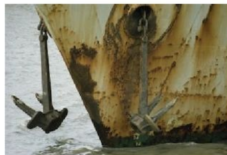
Ships' hulls have to be painted regularly, otherwise they will succumb to rust from contact with salt water and air.
