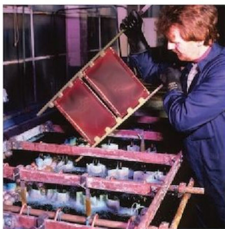
Copper-plated sheets being removed from an electrolysis cell containing copper(II) sulfate electrolyte
