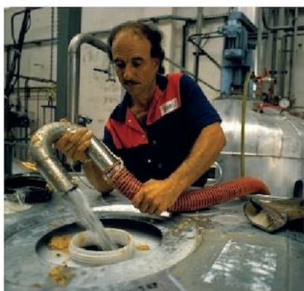
Jasmine oil is extracted by adding water to jasmine flowers and distilling off the oil
