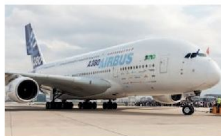
Aircraft bodies are made from alloys of aluminium because these alloys are strong yet lightweight
