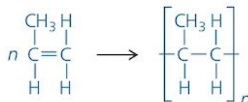
Figure 19.2.2 The repeating unit for poly(propene) from a large number ( n ) of propene monomers
