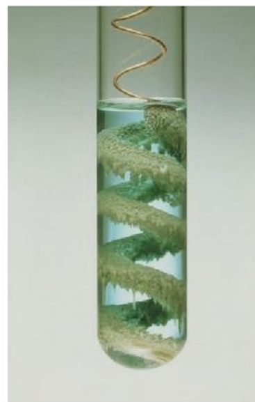
The copper has reacted with silver nitrate and crystals of silver have formed on its surface
