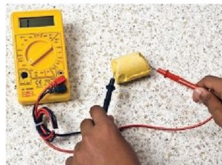
Testing an element for electrical conductivity
