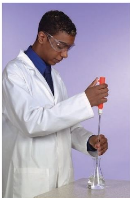
Using a volumetric (graduated) pipette
