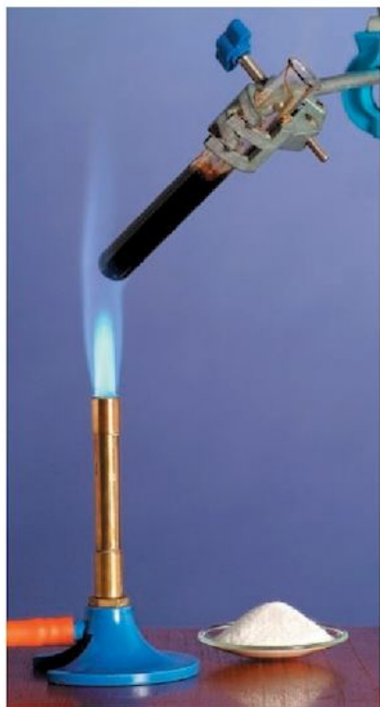
Most organic compounds char or burn when heated in air. Most inorganic compounds just melt or vaporise.
